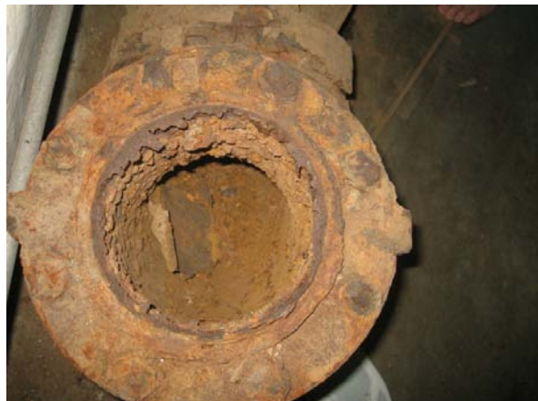
Recently removed pipes and valves – not amount of corrosion
