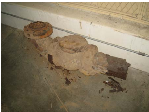
Recently removed pipes and valves – not amount of corrosion
