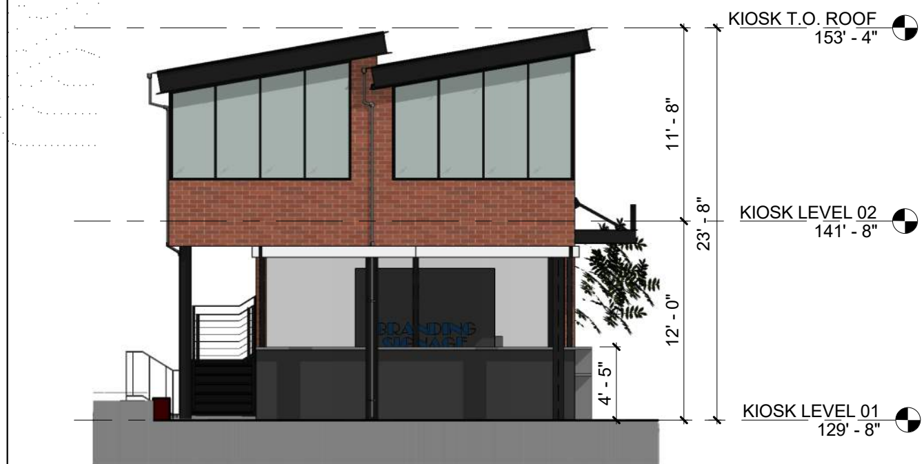
1 KIOSK - EAST ELEVATION DA 1/8" = 1'-0"
