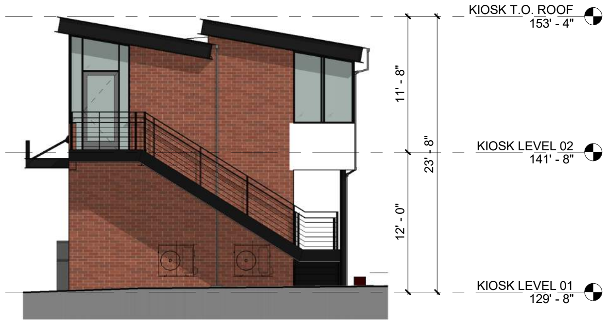
4 KIOSK - WEST ELEVATION DA 1/8" = 1'-0"
