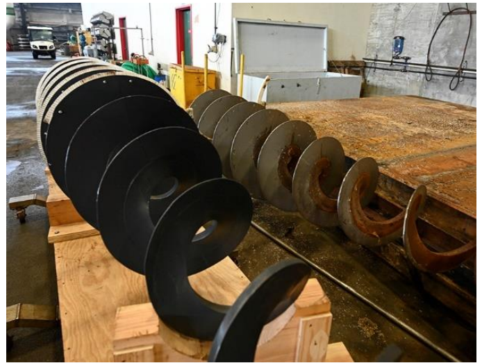
Figure 15: Internal screws from the spiral lifts, out for maintenance.
