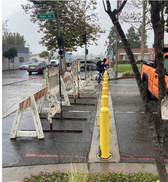
Figure 18 - Bollard receptacles on Main Street, which allow the segment to be temporarily closed, in this case, for a farmers market
