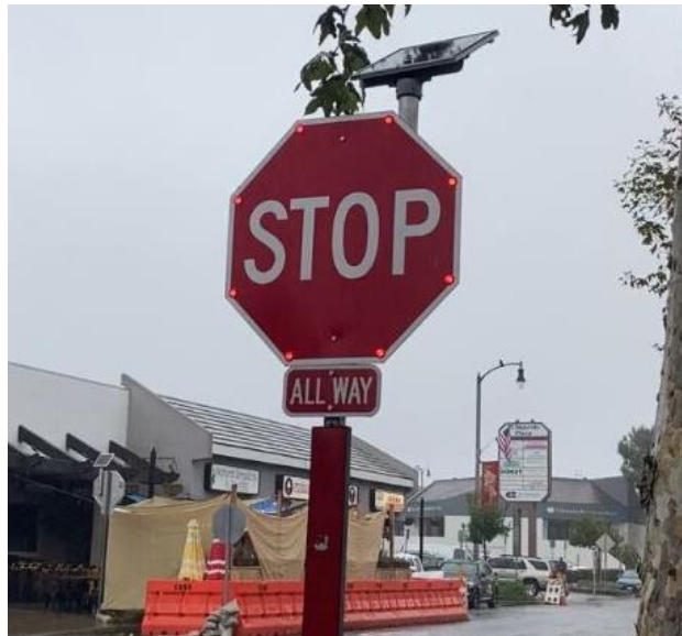
Figure 2 - LED flashing stop sign at the intersection of Main Street and Franklin Avenue
