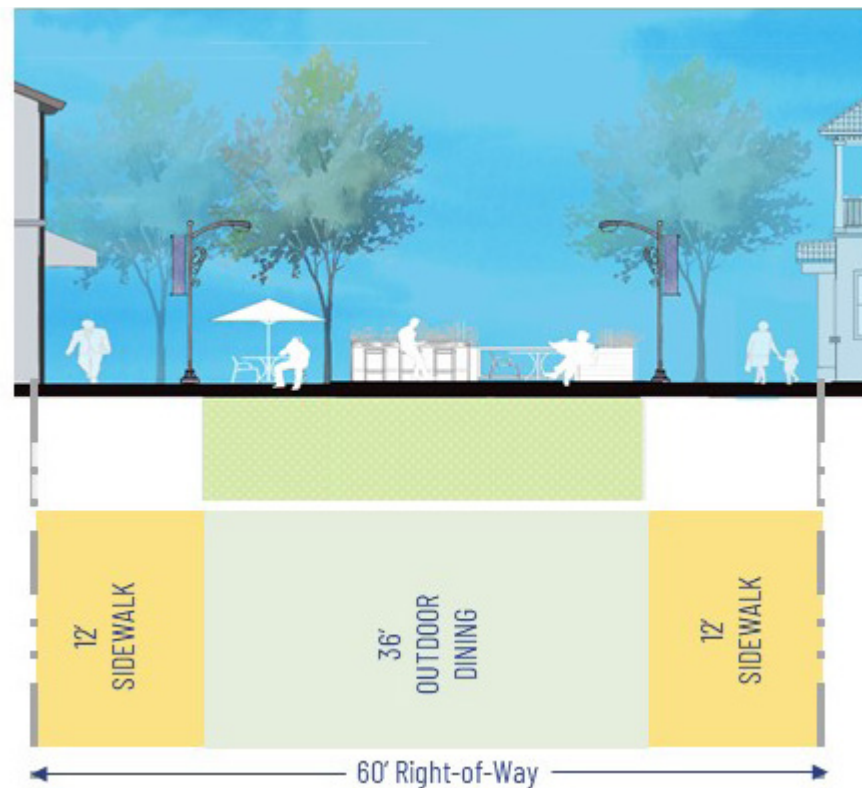
Figure 3.15 Richmond Street Alternative Road Section
